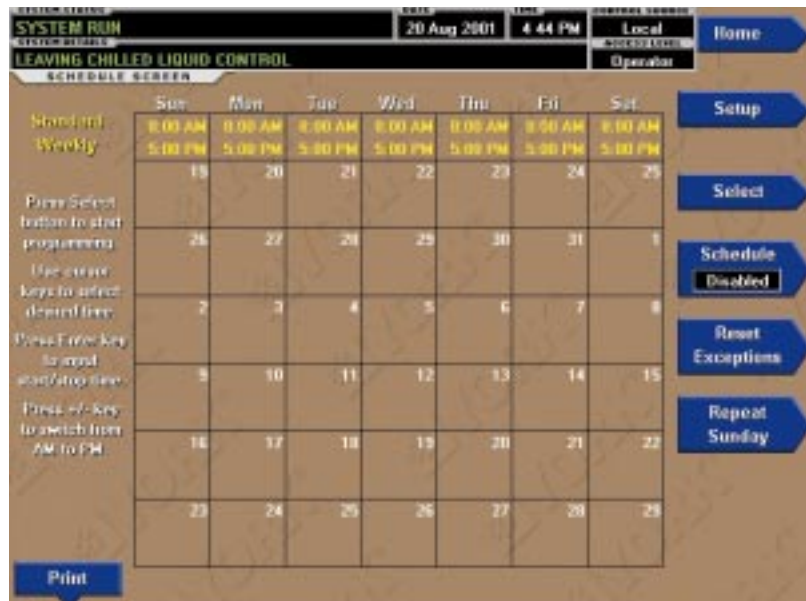
The OptiView Control Center helps you operate your chiller more efficiently by allowing for the precise setting of chilled-water temperature and operating schedule.
