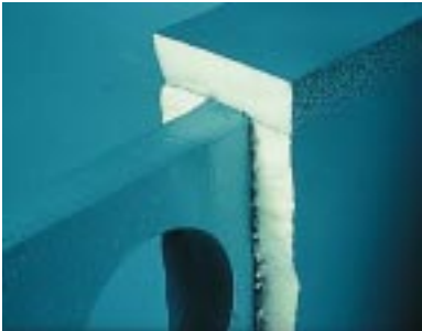
Antisweat insulation can be factory applied.
