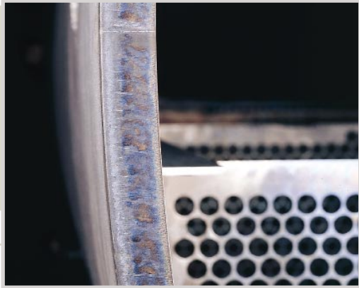
To withstand the demands of higher operating pressures, Titan chillers feature heavy-gauge shells.
