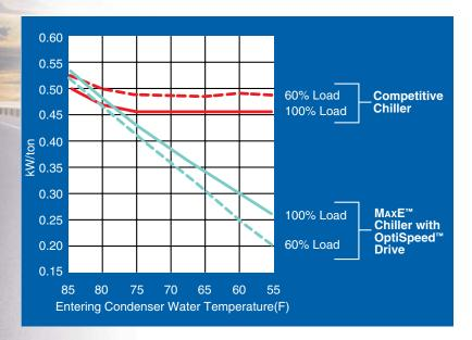
Unsurpassed in energy efficiency, MaxE centrifugal chillers can reach 0.20 kw/TR at off-design conditions.
