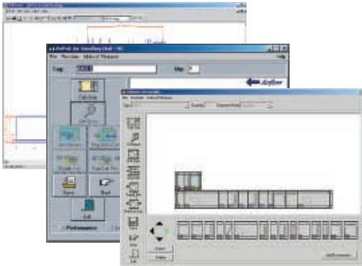
Using the YORKworks program, our sales engineers can select and configure Solution AHUs, draft specifications, prepare schedules, and produce AutoCAD® drawings right on their computer. For highly complex configurations or performance requirements, a team of factory engineers are available to support our sales engineers.
